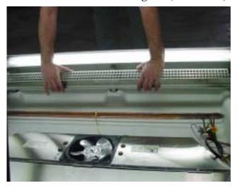
STEP 8 – Rotate fan plenum up and back; hook chain at rear of liner.
